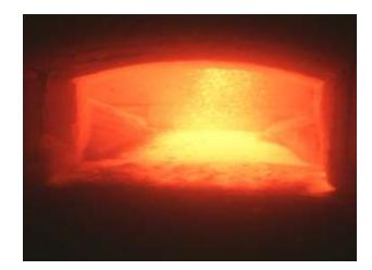
Coanda effect adds transport capacity to the clinker bed avoiding special blaster
