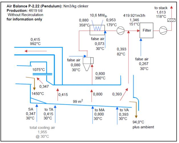
IKN...cool down Case Study-2 Partial recirculation of cooler vent
